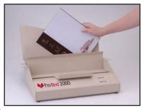
2 Place the cover in the Pro-Bind 2000 machine as shown. You can bind up to 10 documents at one time.
