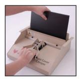
Place Hard Cover into Crimper to crease spine and complete the binding process.
